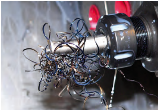
Optimization of process parameters – an example of critical chip formation
