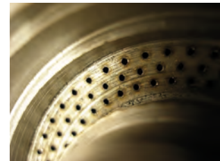
Holes by laser drilling
