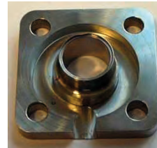
Technology optimization of the specific part resulted in 5× higher productivity and better surface quality
