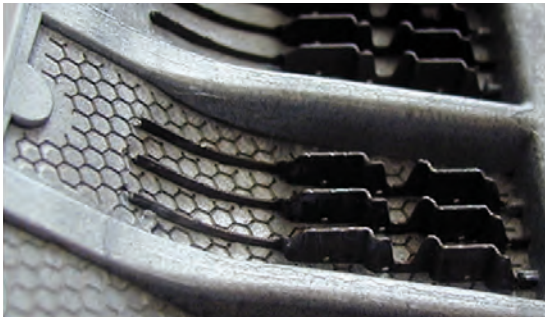
Laser texturing of the mold
