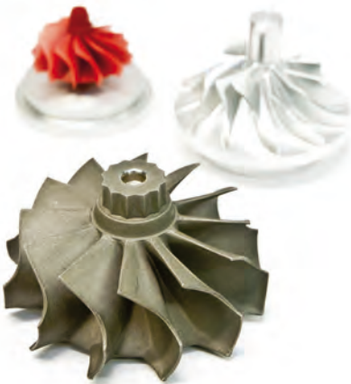
A wax model of a gas microturbine and the resulting casting
