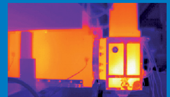
Research of machine tool thermo-mechanical behavior, minimization and compensation of thermal errors
