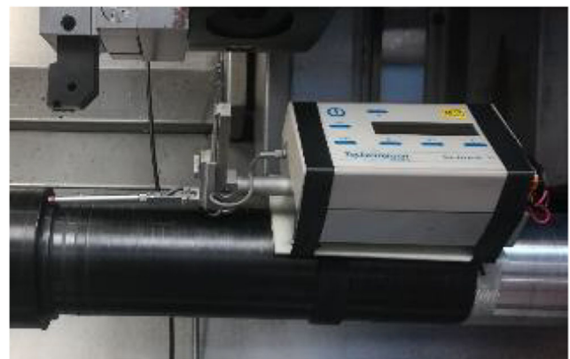
Fig. 7 Surtronic 3+ - Surface roughness measurement
