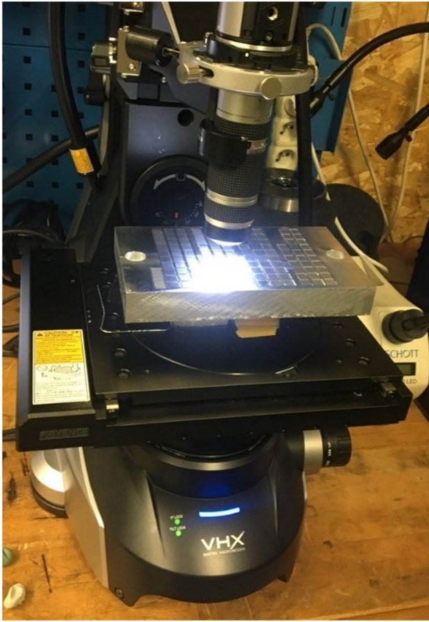
Fig. 7 Optical surface measurement (using the KEYENCE microscope)
