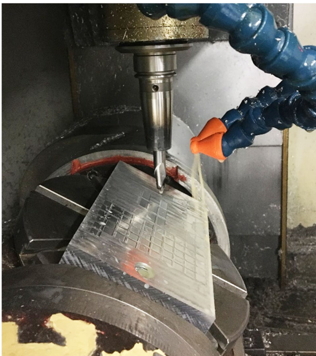
Fig. 5 Milling experiment (tool D12)
