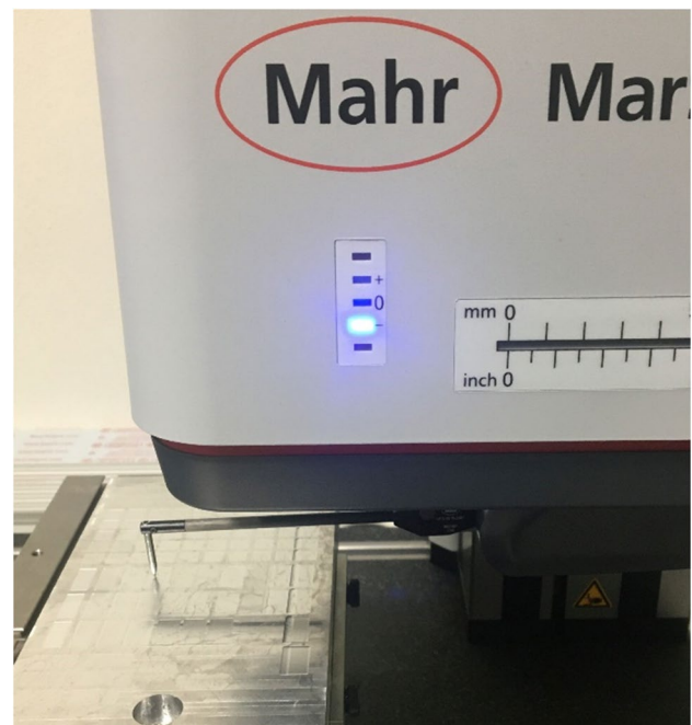
Fig. 6 Surface roughness measurement on the sample (using the Mahr instrument)
