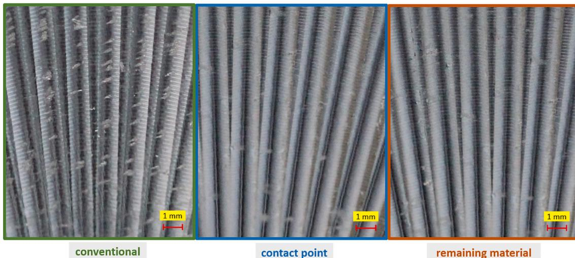
Fig. 22. Detailed comparison of surfaces (machined by three approaches).
