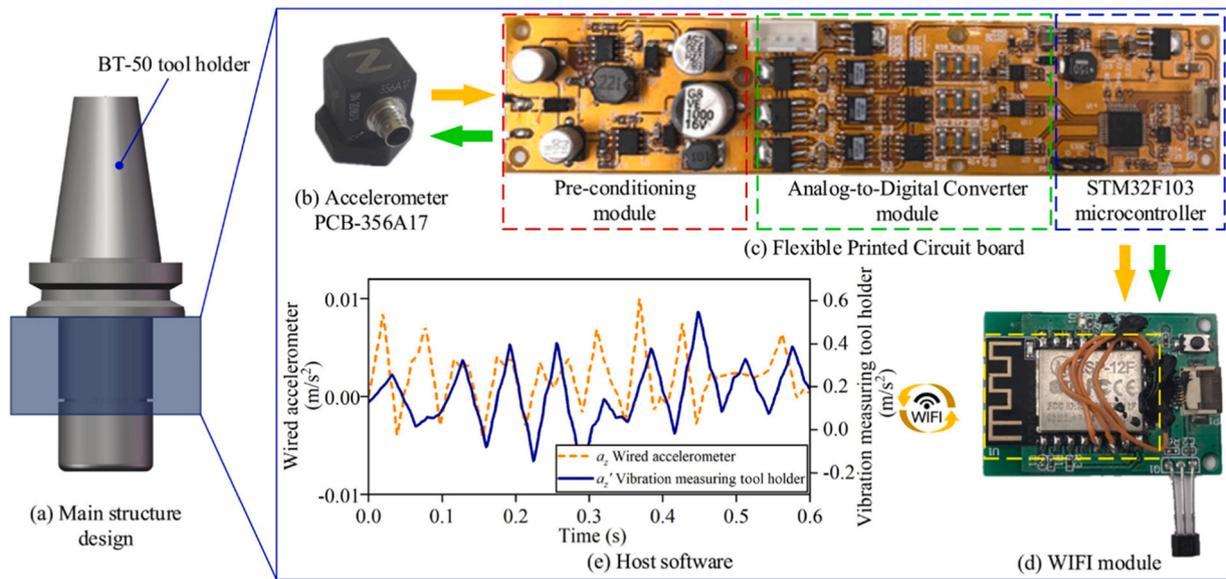
Fig. 42. Wireless communication for a tool holder using STM32F103 microcontroller and a WIFI module [27].
