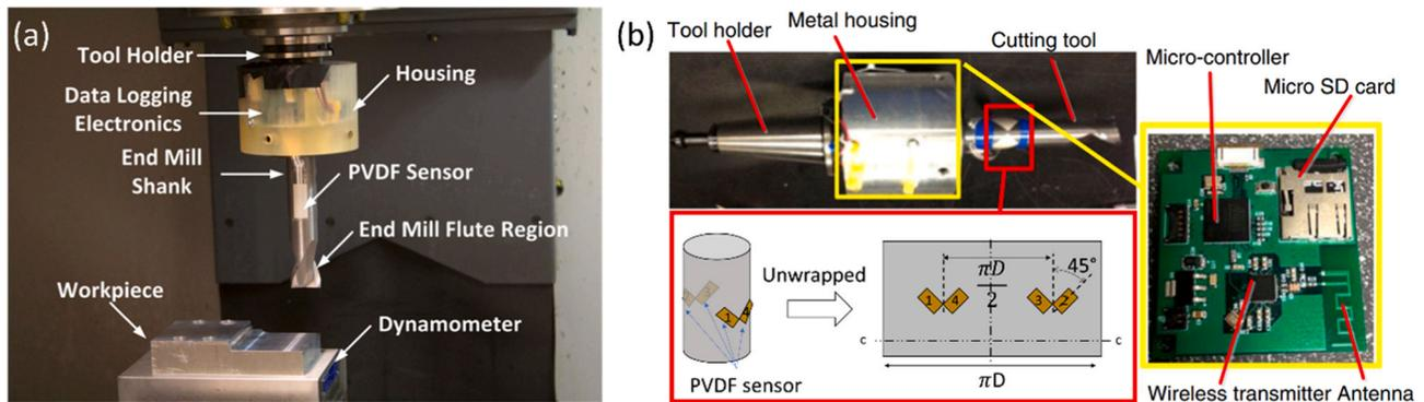
Fig. 12. Tool integrated sensor system proposed by Ma et al. [114,115] for the measurement of (a) feed and transverse forces; (b) cutting torque.
