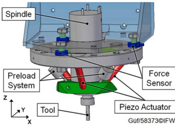
Fig. 29. Adaptronic spindle system (AdSpin) [173].
