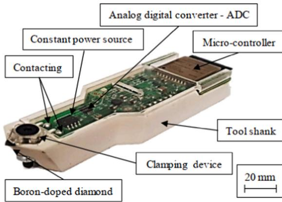
Fig. 11. A nanocrystalline diamond-based multilayer wear sensor system [111].
