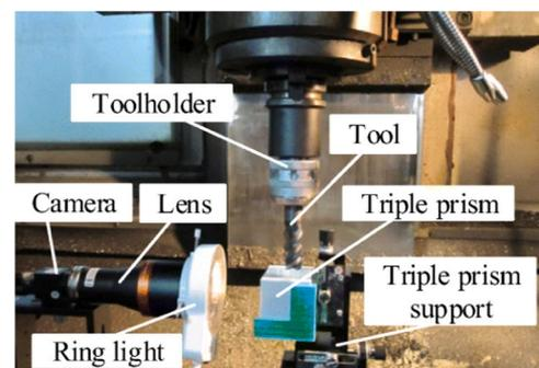
Fig. 6. Vision system for on-machine tool wear measurement [93].
