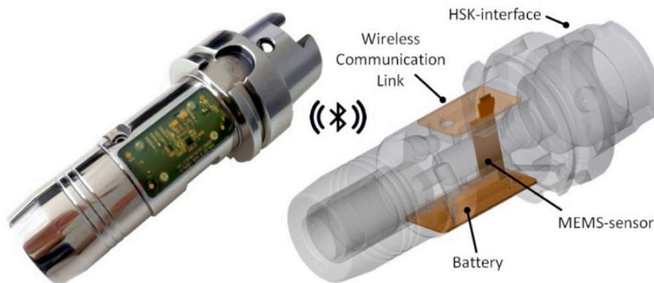
Fig. 22. Uniaxial MEMS accelerometer in tool holder developed by Bleicher et al. [141].
