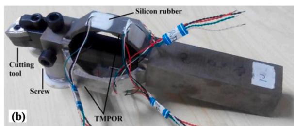
Fig. 25. High-sensitivity strain gauges used by Zhao [151,152]: (a) semiconductor strain gauges; (b) MEMS strain gauges.
