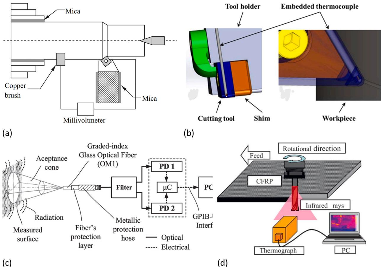
Fig. 4. Example sensor placement/configuration of (a) tool-work thermocouple [50], (b) embedded thermocouple [51], (c) infrared pyrometer [52], and (d) infrared camera/thermograph [53] for cutting temperature measurements.
