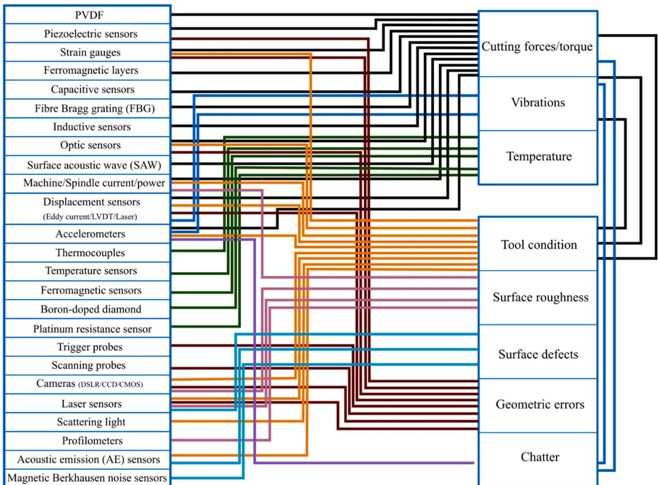
Fig. 1. Summary of the types of sensors discussed in this paper for direct and indirect measurement and monitoring of various parameters during machining.
