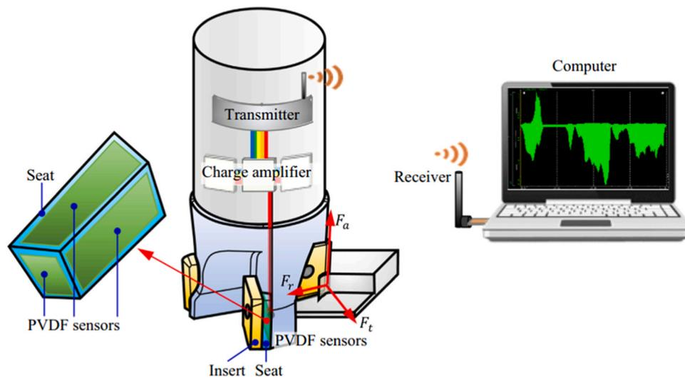
Fig. 14. Embedded PVDF sensors into the seat of each cutting insert developed by Luo et al. [119].
