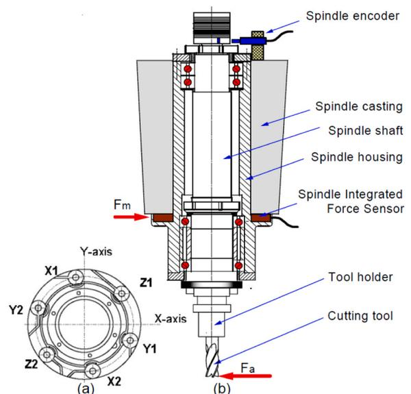
Fig. 28. Assembly of the force sensors between the spindle and the spindle stock: (a) top view, (b) schematic cross section [170].
