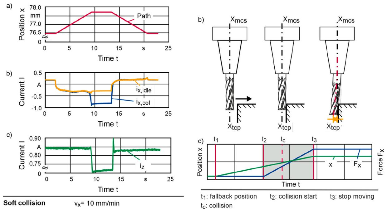
Fig. 38. Principle of the system stiffness identification using the drive current and axis position measurement [191].
