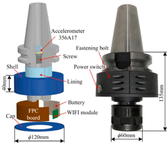
Fig. 23. Three-axis accelerometer in the tool holder designed by Zhou et al. [27].
