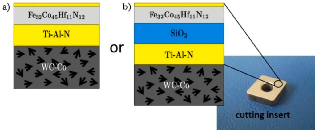
Fig. 10. Sensor layers consisting of SiO<sub>2</sub> and/or Ti-Al-N between the Fe-Co-Hf-N sensing layer and the WC-Co substrate [109].
