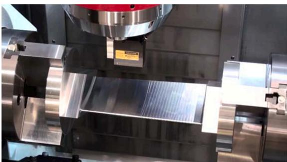
Fig. 5. laser displacement sensor for freeform profile measurement [81].
