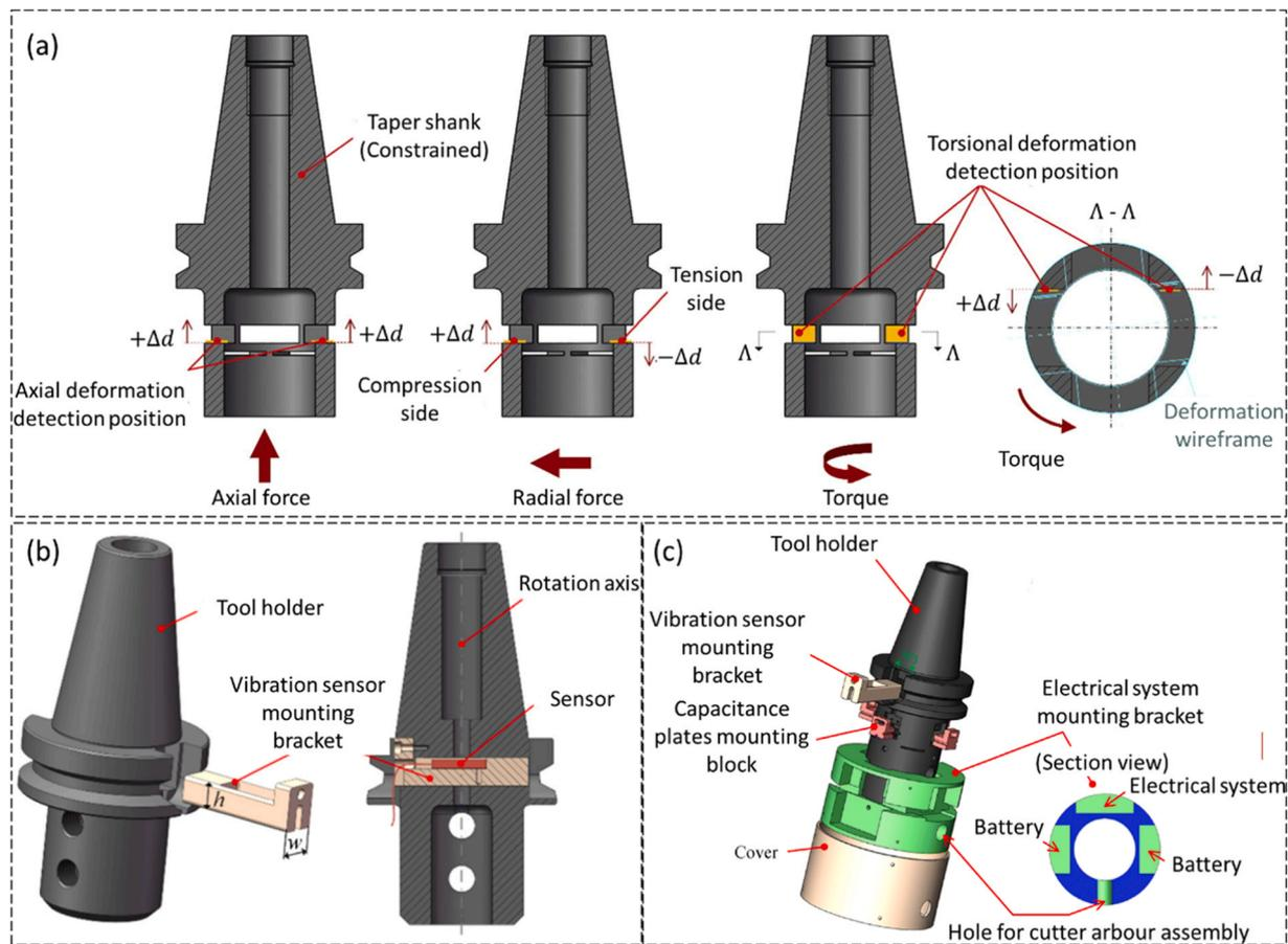
Fig. 21. Modified tool holder by Xie et al.: (a) cutting force sensors [134]; (b) cutting vibration sensor [135]; (c) multi-sensor [136].
