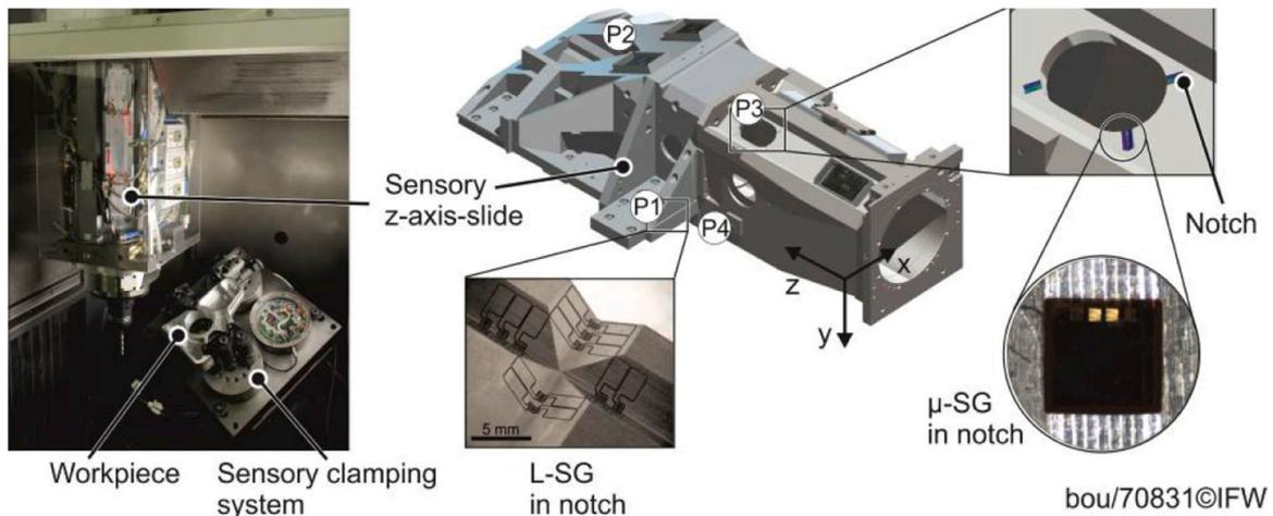
Fig. 31. Example of the Z-slide of a vertical milling centre with integrated strain gauges located in four positions (P) [175].
