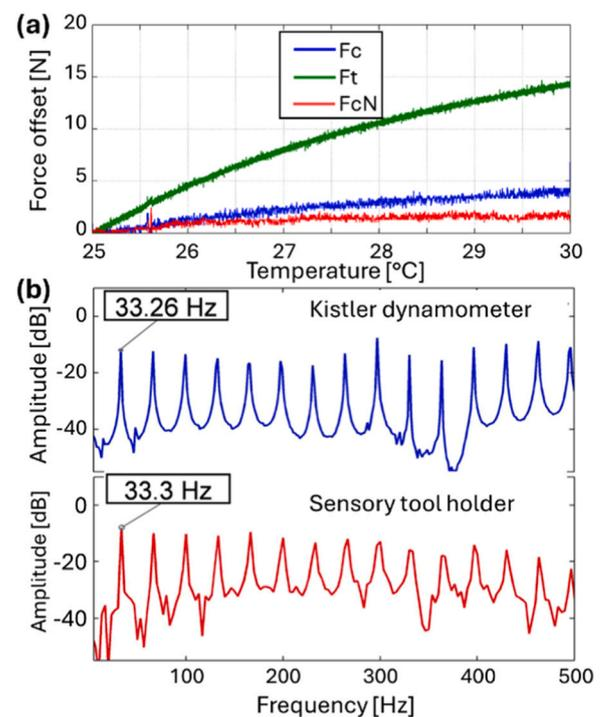
Fig. 18. (a) Impact of temperature on the force measured by the multi-sensor integrated tool holder [129] and (b) comparison of forces measured by a Kistler dynamometer with multi-sensor tool holder [28].
