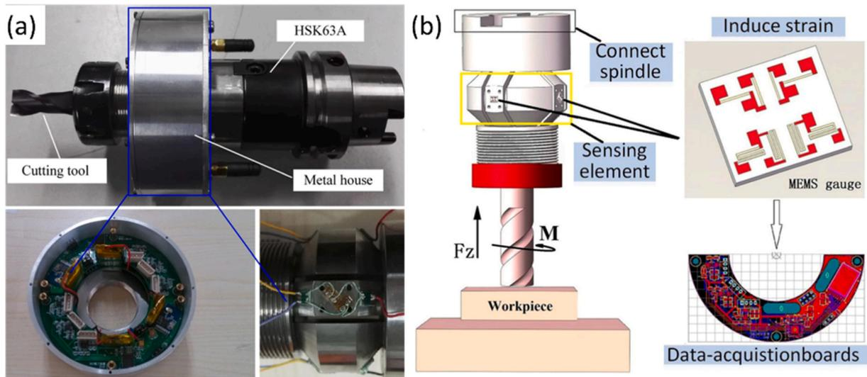
Fig. 20. MEMS strain gauges integrated in the tool holder to measure (a) axial force and torque [131] (b) torque [133].
