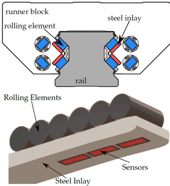
Fig. 32. Position of steel inlays (red) below the rolling elements (blue) inside the linear guideway carriage and sketch of the sensor position on the steel inlay [178].
