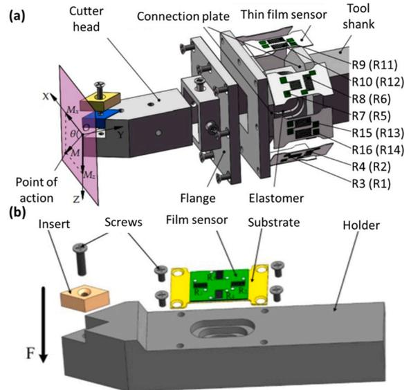
Fig. 26. Thin-film strain sensors integrated in the turning holder: (a) Zhang [153]; (b) Cheng [154].
