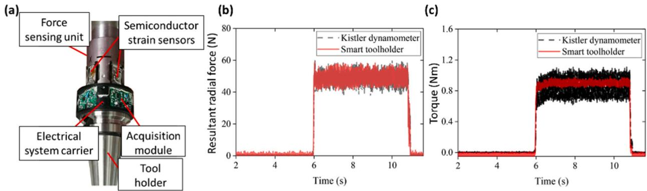
Fig. 19. (a) smart tool holder with semiconductor strain gages and a comparison of (b) resultant radial force and (c) torque measured by the tool holder and Kistler dynamometer [130].
