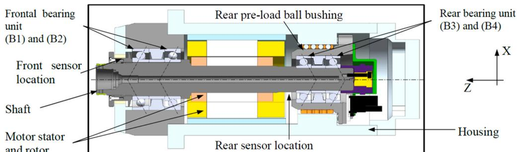
Fig. 43. Electro-spindle components (without tool and tool holder) [228].
