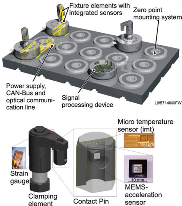
Fig. 33. Sensory fixture with strain gauges and MEMS accelerometer integrated in the clamping element [180].
