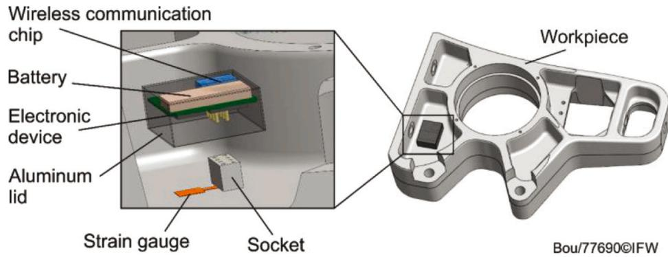
Fig. 35. Concept of the low-cost sensor for integration to the workpiece [185].
