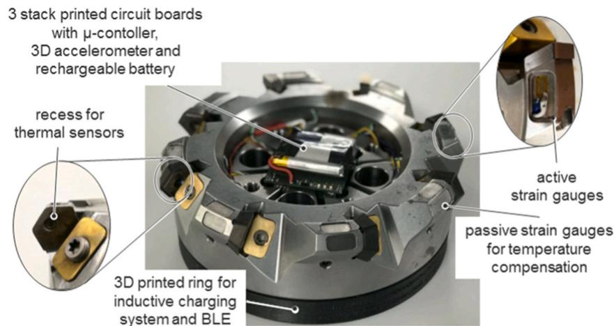
Fig. 16. A prototype milling tool integrated six strain gauges, K-type thermocouples, an MEMS accelerometer and position sensor [123].
