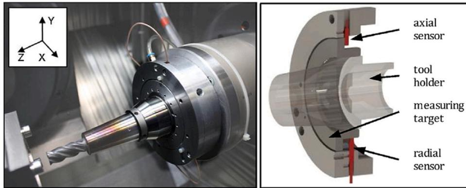
Fig. 30. Integration of the sensory ring with eddy current sensors into the electrospindle design [174].
