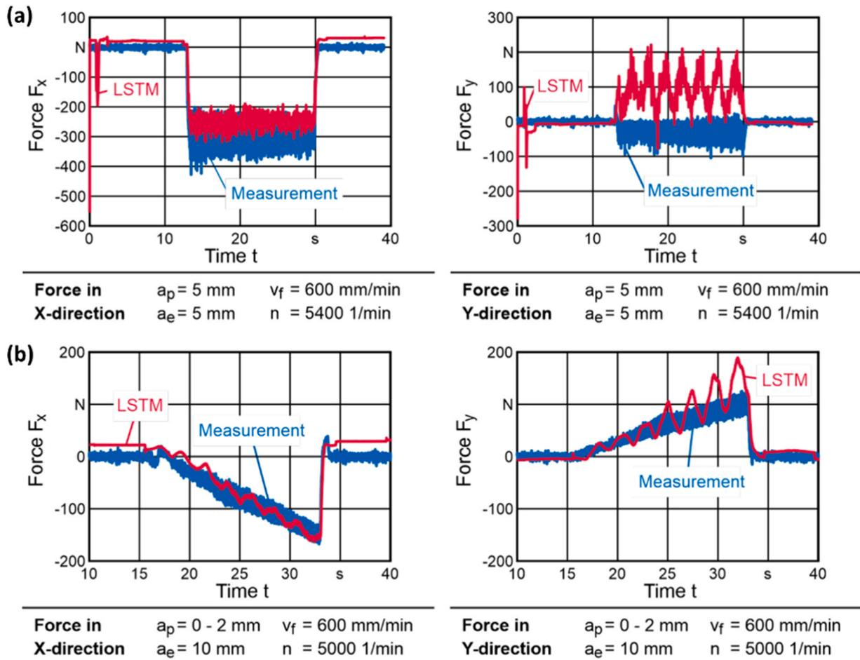
Fig. 37. Measured cutting forces in x and y direction against predicted values using LSTM for two machining scenarios: (a) side milling in negative X direction and (b) ramp milling in negative Y direction and positive Z direction.
