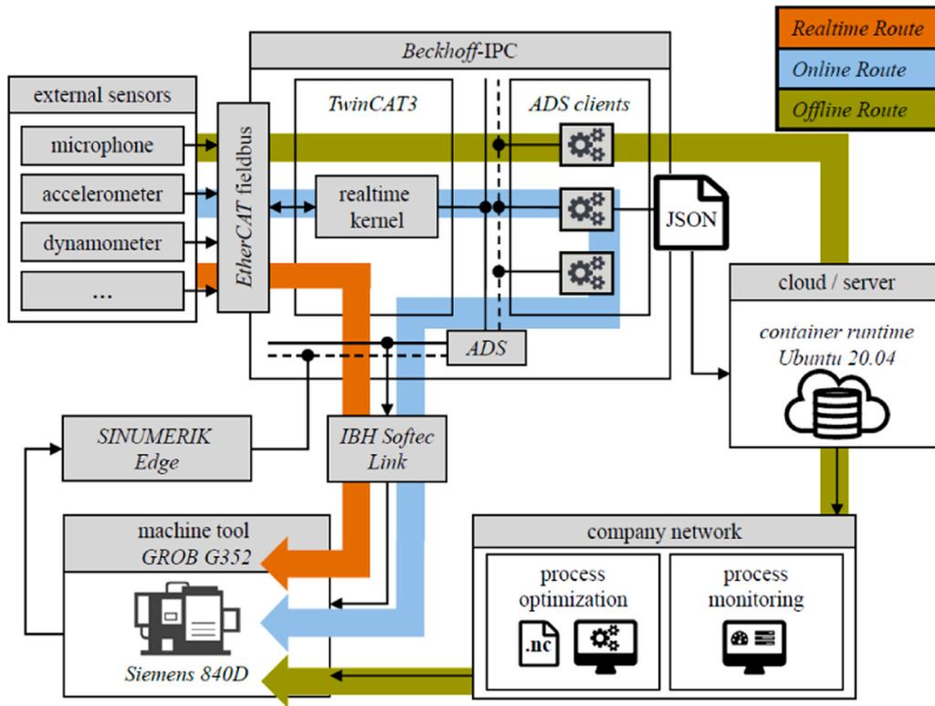
Fig. 40. Process monitoring and control platform with highlighted real-time, on-line and off-line processing routes [203].
