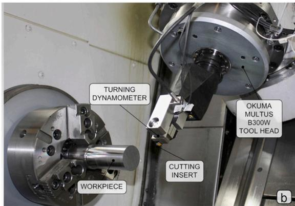
Fig. 24. A piezoelectric force ring assembled on the turning tool holder [146].
