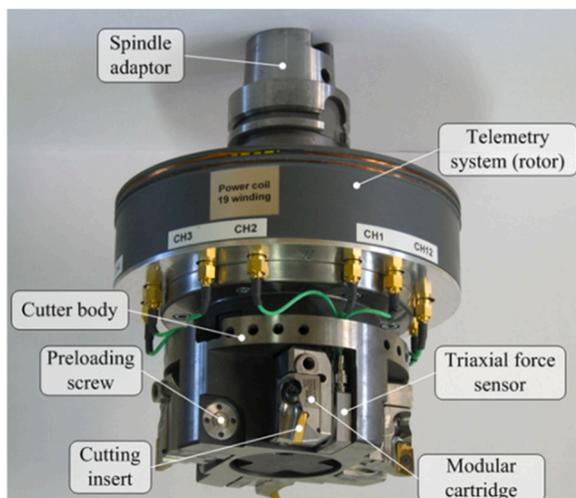
Fig. 17. Rotating dynamometer proposed by Totis et al. [3].
