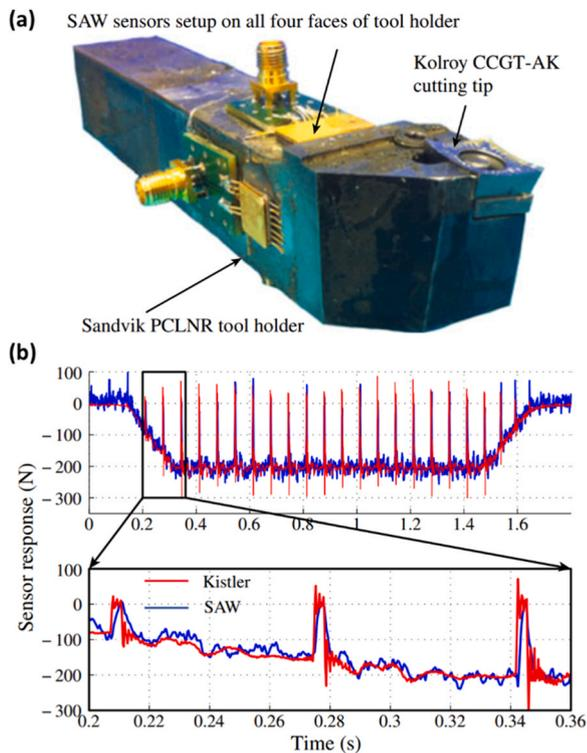
Fig. 27. (a) SAW strain sensor integrated in the turning tool holder and (b) example cutting force signal from the tool holder compared with Kistler dynamometer in dual axis oblique interrupted cutting [155].
