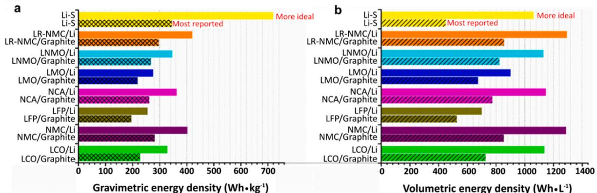
Fig. 41. a) Gravimetric and b) volumetric energy density of various batteries [205].
