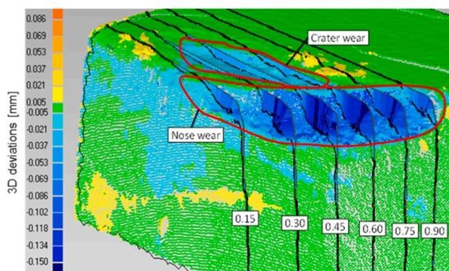
Fig. 7. Reconstructed 3D model of a worn cutting edge [100].
