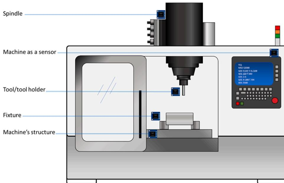
Fig. 2. Potential sensor locations for on-machine in-process monitoring and measurement.
