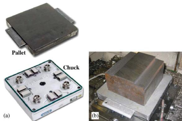
Fig. 34. Sensory pallet with active vibration avoidance: a) the pallet (upper), chuck permanently fixed a machine table (lower); b) the pallet system equipped with a steel workpiece [181].
