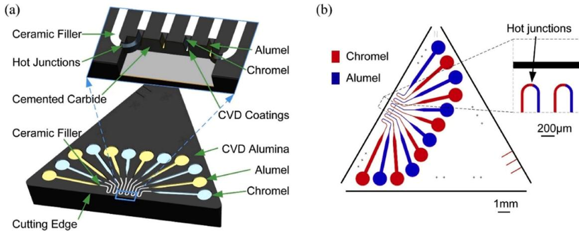
Fig. 8. (a) Schematic of the embedded distributed pattern of thin-film thermocouples and (b) its horizontal view [103].
