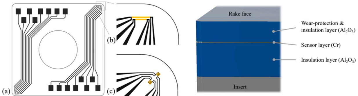
Fig. 9. Direct deposition of the layers in the sensor on the rake face of the uncoated cutting tool [108]: (a) overview of the sensor, (b, c) sensing zones.
