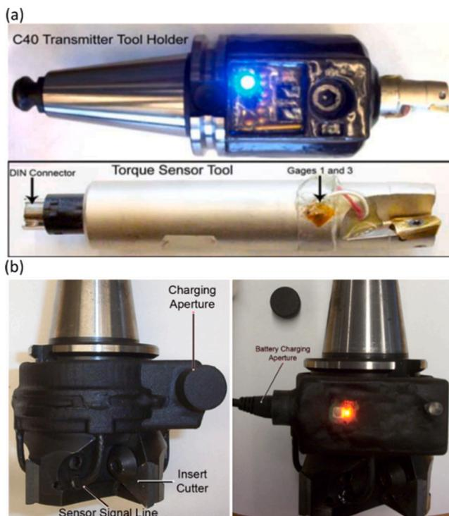
Fig. 15. (a) Cutting torque and (b) tool tip vibration measuring system [120,121].
