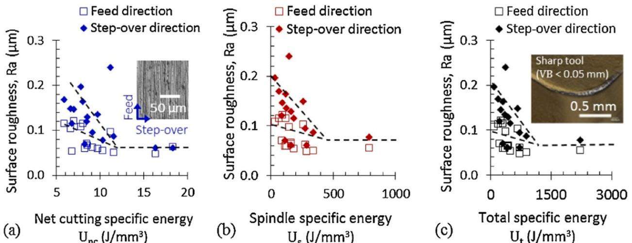
Fig. 39. Coherence of surface roughness with (a) specific cutting, (b) spindle, and (c) total specific energy by milling with a sharp tool ( $VB < 0.05$  mm) [193].
