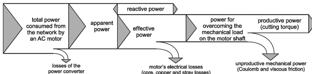
Fig. 36. Power flow in a motorized spindle – an overview of various types of power losses [187].
