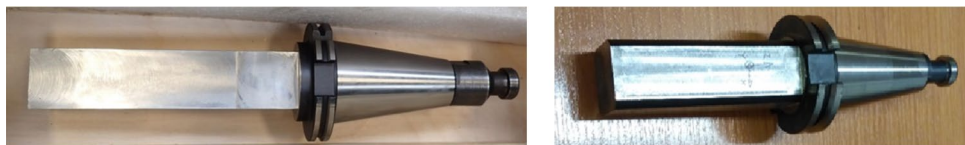
Fig. 7 Artifacts 45 \times 45 \times 200 mm for WHT 110 (left) and 32 \times 32 \times 100 mm for MCFV1260i (right)
